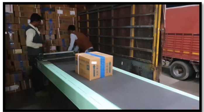
TBC unloading directly inside the container – Making it easy for the operator
