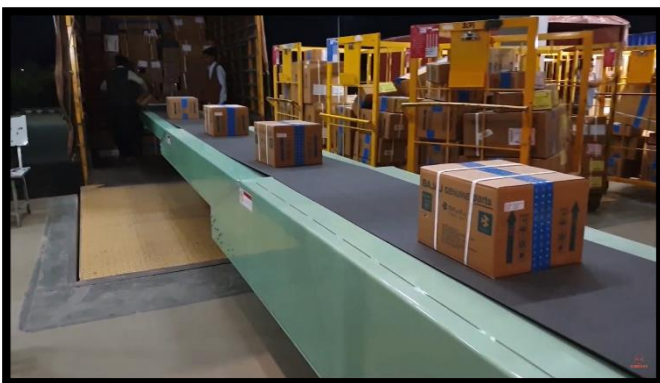
TBC unloading directly inside the container – Making it easy for the operator
